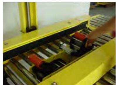
Check tape cutter position and adjust as needed.
