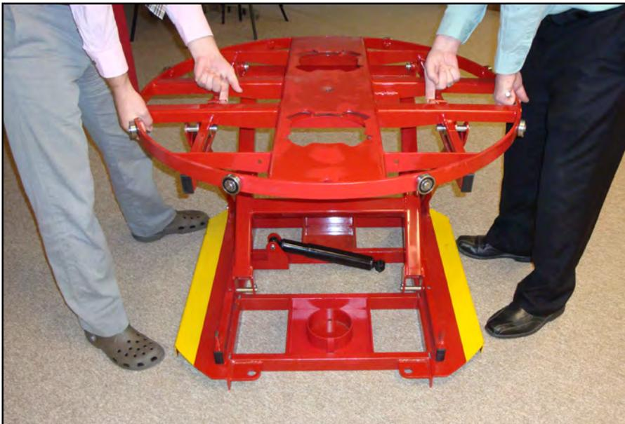
4. With the help of an assistant, lift the top frame until it hits the upper latch stops.
