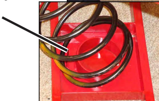
6. Insert either end of the large orange spring into the lower pocket. Be sure the bottom spring coil is positioned outside the alignment tab as shown.
